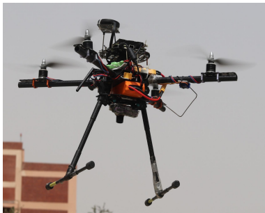
(a) MAV-1: A system with heavy payload carrying capabilities, equipped with Intel NUC and VIO sensor
