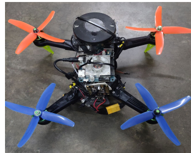
(b) MAV-2: A system capable of high speed surveying equipped with RTK-GPS and a high resolution camera
