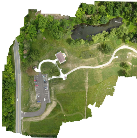
Figure 10: 2D RGB map using ODM, this map was created in 45 seconds using 8 individual images
