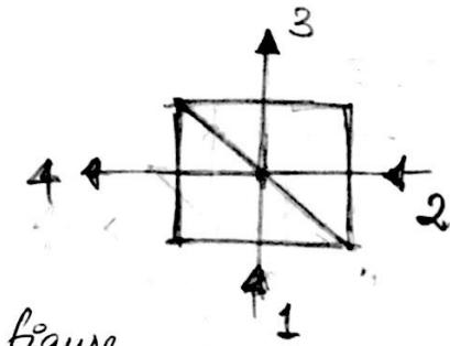
$$\vec{E}_3 = T_{13} \vec{E}_1 + R_{23} \vec{E}_2 \quad \text{(transmitted)} \quad \text{and} \quad \vec{E}_4 = T_{24} \vec{E}_2 + R_{14} \vec{E}_1 \quad \text{(transmitted)}$$
