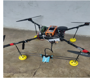
(c) MAV-3: A system capable of detection and delivery, equipped with NVIDIA Jetson TX2, OCam and servo grippers
