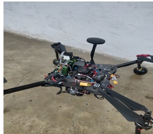
(b) MAV-2: A system capable of high speed surveying equipped with RTK-GPS and an OCam Camera
