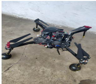
(a) MAV-1: A system with heavy payload carrying capabilities, equipped with NVIDIA Jetson TX2
